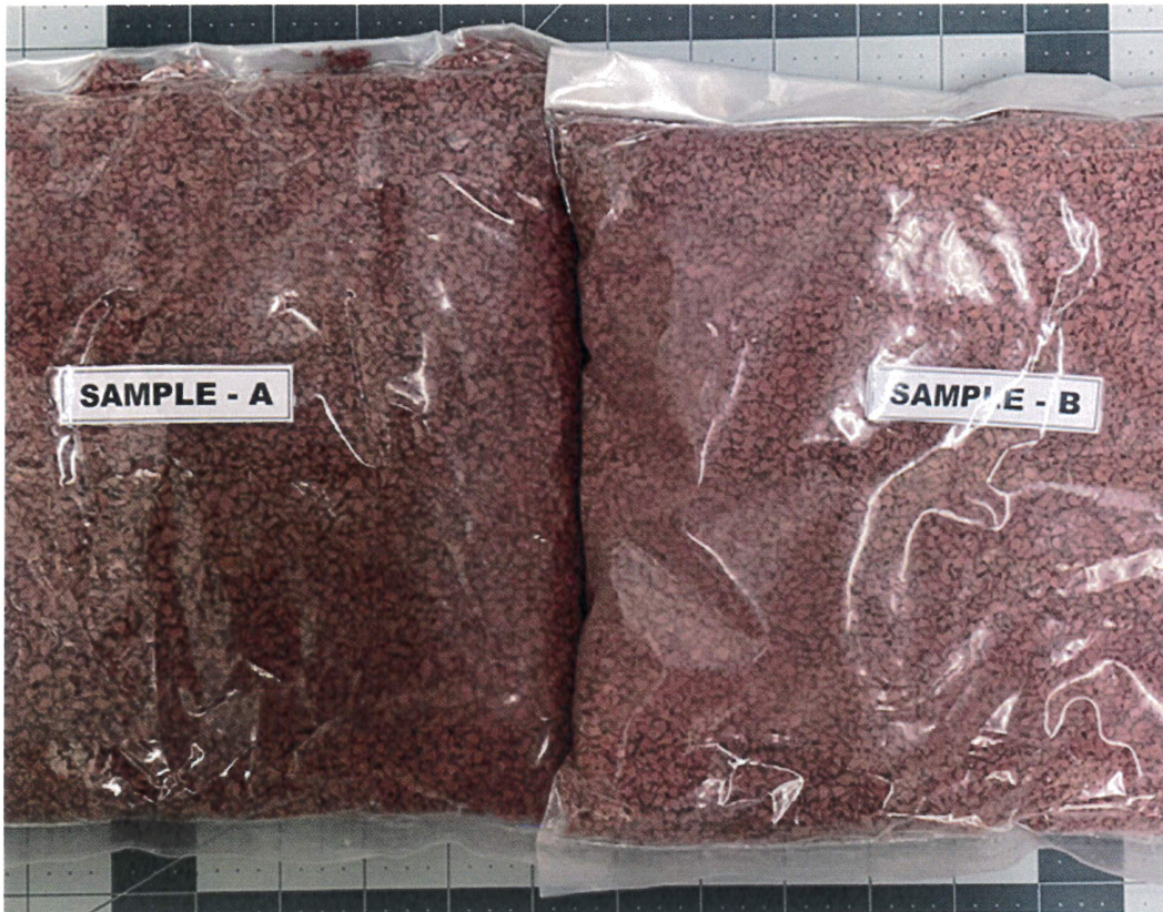
Two (2) Intact Bags of Red EPDM Rubber Granules ID as Sample - A & Sample - B
